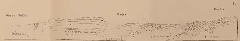
Fig. 3 Section between Kandia and the Morne Nullah
